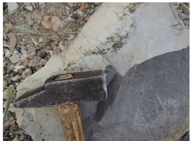
Fig. 5 Variety of Pietra Alberese named sasso porcino , dark grey in the fresh cut
