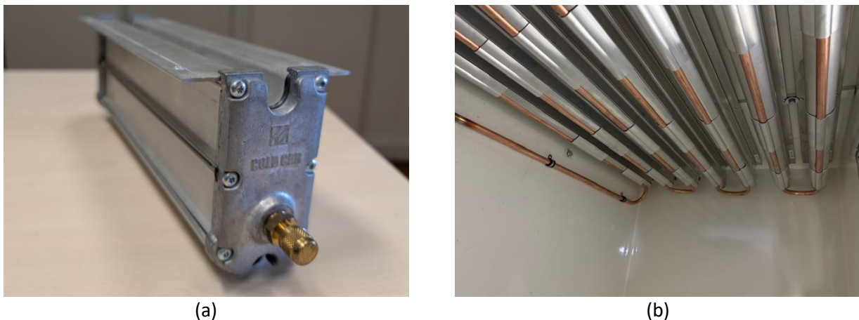
Figure 2. Eutectic tubes: (a) front view detail; (b) complete tubes setup inside the insulated box.
