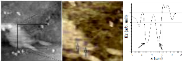
Fig. 1. (Left), 20\mu\text{m} \times 20\mu\text{m} topography of h9c2 mouse cell recorded with a home-made aperture SNOM; (middle) an overlapping of the topography image with the correspondent optical map, the arrows denote the NS identified within the cell; (right), strong-absorption points marked by arrows in the overlapping image and denoting the dimensions of the NSs. (Adapted with permission from [10]).
