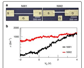
**Fig. 1 a** Scanning electron microscopy (SEM) images of InAs NW field-effect transistors labelled NW1 and NW2, with source (S), drain (D), and gate (G) contacts indicated. **b** The conductivity  $\sigma$  of NW1 (black line) and NW2 (red line) measured at room temperature applying drain-to-source voltage of  $V_{DS} = 2$  mV for NW1 and  $V_{DS} = 5$  mV for NW2, reported as a function of the gate voltage  $V_G$ .
