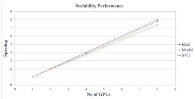
Fig. 4. Speedup curves of the algorithms implemented on GPUs within the FR P-SBAS processing chain. In particular, the blue linear behavior represents the ideal speedup, whereas the orange and the grey curves show the measured speedups relevant to Step B and Step C of the processing chain (see Fig. 2), respectively, as described in Section IV.
