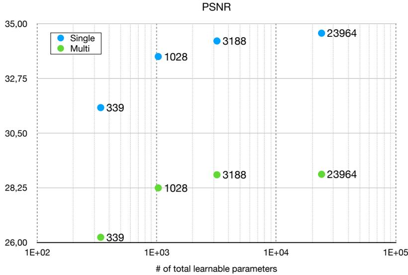
Figure 3: Average PSNR vs number of parameters on SynthRTI. The x-axis is in logarithmic scale, so to show the benefit from choosing a configuration with less parameters.
