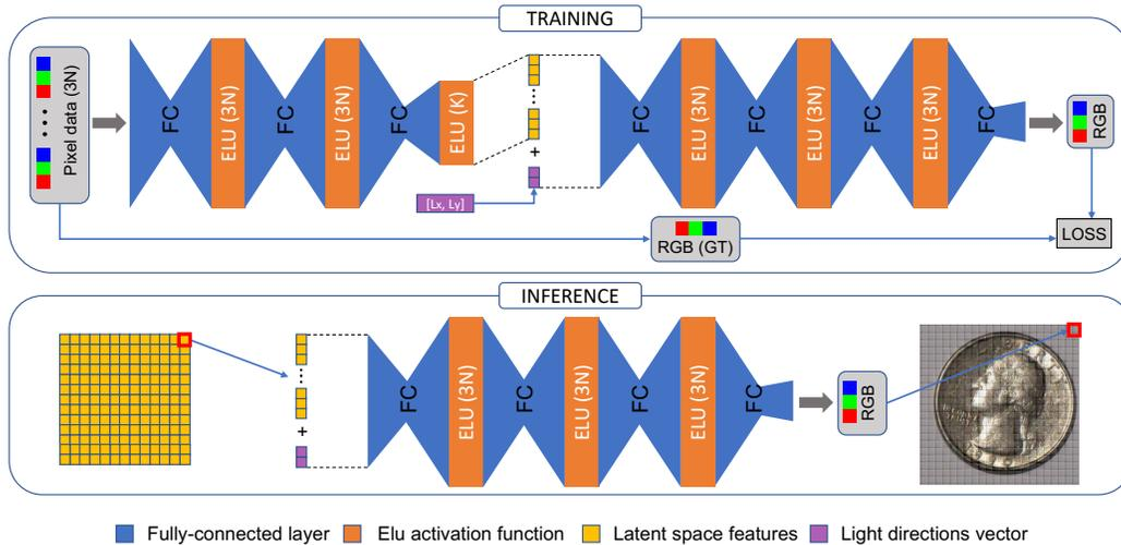
Figure 1: Original NeuralRTI scheme.<sup>4</sup> Top: training network with the encoder (3 layers) and the decoder (4 layers). They have the same number of parameters set to  $3N$ . Bottom: the relighting (inference) is made with the decoder only starting from the saved latent space features (stored as image layers) and creating the RGB values for all the image pixels given an input light direction
