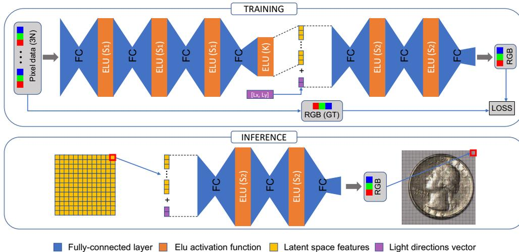
Figure 2: Modified NeuralRTI scheme. Top: training network with the encoder (4 layers) and the decoder (3 layers). They can be tuned in different ways. Bottom: inference, using the decoder only given the latent features layers and the novel light direction. Note that the size of the decoding layers can be configured (setting it as desired in the training phase and storing the information as an input for the shader).
