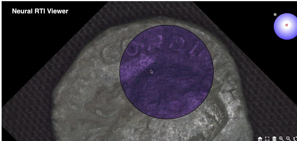
Figure 5: Video 1, showing the interactive tool for RTI-based coin analysis. The surface can be relighted from controlled directions, the view can be rotated and zoomed and the lens options can show different layers (in the examples normal map and relightable UV image). <http://dx.doi.org/doi.number.goes.here>
