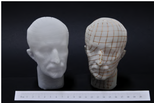
Fig. 2. Photo of the 3D printed prototype for the MAX PLANCK model. Next are the renderings of the 3D model used for printing, the internal pipes, and the bottom part of the model with the exits of the sensor conductors.
