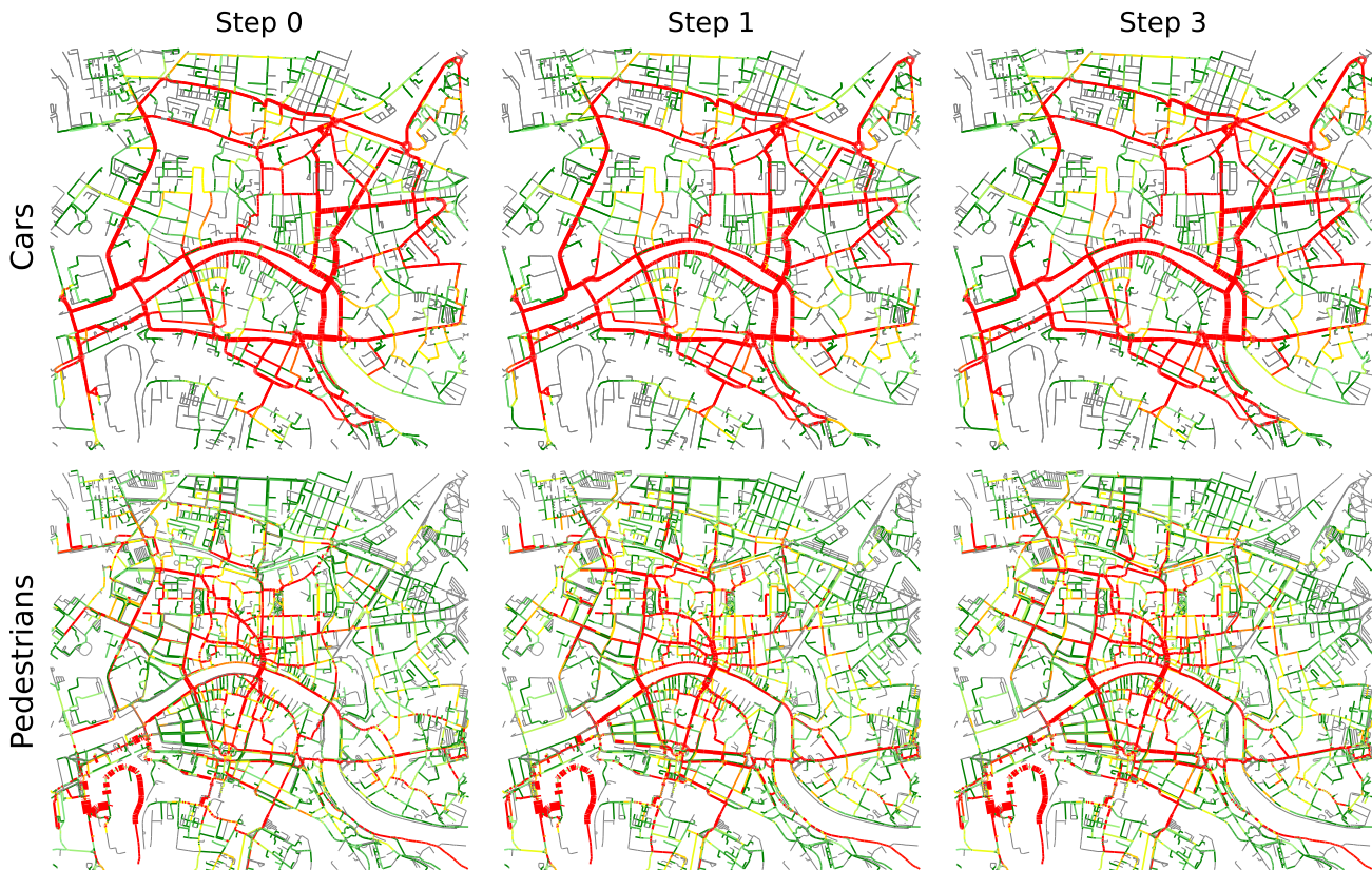
Fig. 8: Road usage evolution for cars (top) and pedestrians (bottom) at simulation steps 0, 1, and 3 using local weighting. Line width and color intensity reflect the square root-transformed traffic volume: thicker, redder lines indicate heavier usage, while thinner, greener lines indicate lighter traffic.
