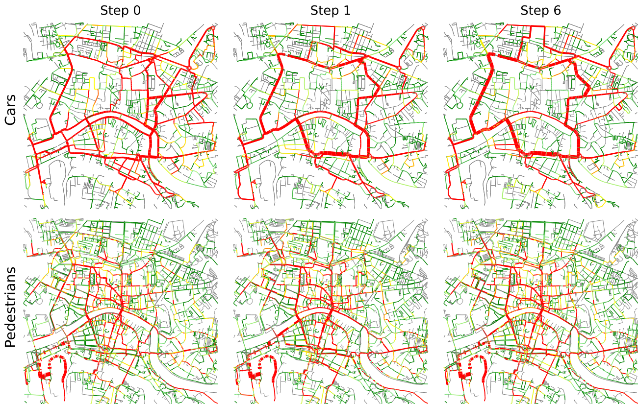
Fig. 5: Road usage evolution for cars (top) and pedestrians (bottom) at simulation steps 0, 1, and 6 using global weighting. Line width and color intensity reflect the square root-transformed traffic volume: thicker, redder lines indicate heavier usage, while thinner, greener lines indicate lighter traffic.
