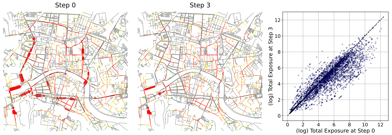
Fig. 10: Evolution of total pedestrian exposure across simulation steps under the local trade-off strategy. The maps (left and center) show exposure per road segment at steps 0 and 3, respectively, where both color and line width indicate the magnitude of exposure (log-transformed). The scatter plot (right) compares log-transformed exposure values between step 0 and step 3, with each point representing a road segment.
