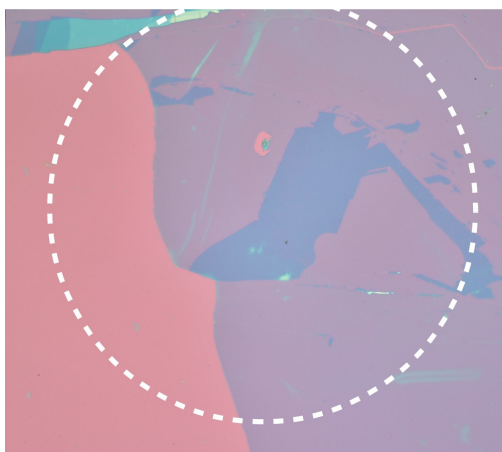
Fig. 2. Reflectivity image of the sample under visible illumination, collected with an optical microscope equipped with an RGB camera. The white dashed circle denotes the area that is illuminated by the laser used for the acquisition of Raman and fluorescence images. The image has been collected with a 10 \times objective.
