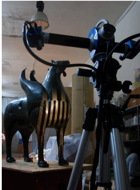
Figure 2: Scanning the Griffin with the Breuckmann SmartSCAN 3D-HE system.
