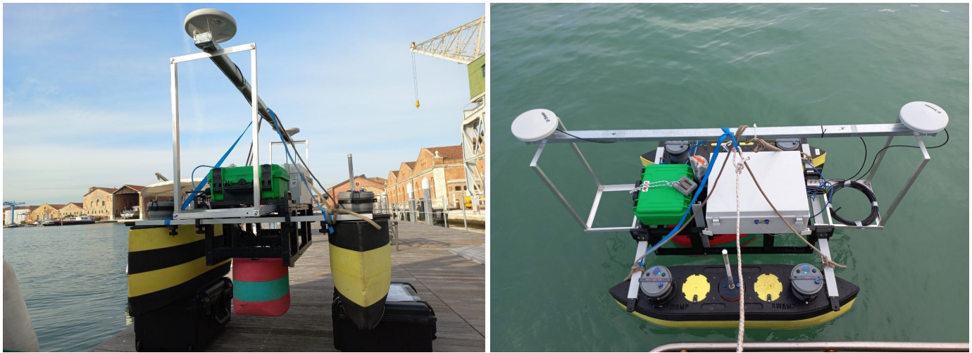
Fig. 1. SWAMP equipped with MBES, two waterproof boxes for Single Board Computer (green) and Sonar interface module (gray), and two GNSS antenna.
