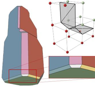
**Fig. 7. Dihedral angles of  $90^\circ$  cannot be obtained using the Marching Cubes algorithm. There will always be small facets as junctions between orthogonal facets. In most of cases, these facets are not suitable for the proposed fabrication task and they could not contribute for a better approximation.**
