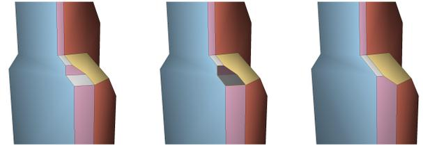
**Fig. 11. Selection and deletion of two adjacent facets.** The facets cannot be deleted singularly due to the adjacency of two facets lying on parallel planes. If selected together, we can close the surface extending the edges of the adjacent facets on the border of the two deleted facets.
