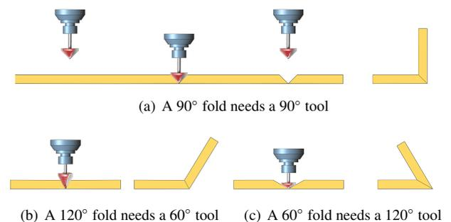
Fig. 3. Different folds made using V-Groove milling tools.
