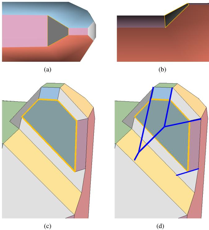
**Fig. 10. Non-removable facets.** In the first row (a) (b), the planes onto which the pink facets lie are parallel and never intersect, so that removing the facet would leave a hole that can not be closed. In the second row (c) (d), the expansion of the contouring facets would produce a mesh self-intersection.
