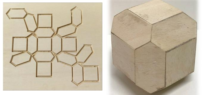
Fig. 22. Manufacturing of a modified sphere. From top left to bottom right: the digital simplified model, its unfolding, the carved sheet of plywood, and a picture of the fabricated model.
