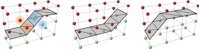
Fig. 6. The configuration on the left is one of our *Masks*. It is a portion of the lattice generating an iso-surface with two facets having normal of type 1 adjacent to a facet with normal of type 2. Switching the signs of the points haloed in blue or orange, respectively, we obtain the configurations at the center and the right. We choose the set of vertices to switch which favors the enlargement of the broader adjacent facet.
