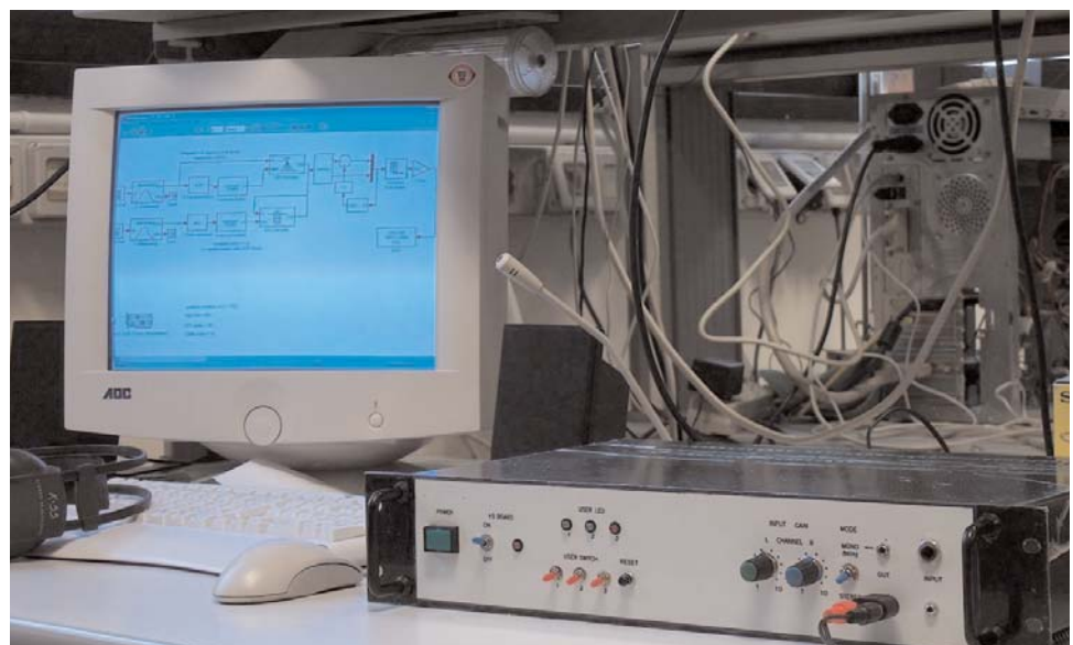
Figure 4. View of the system based on the DSK board, connected to the PC.
