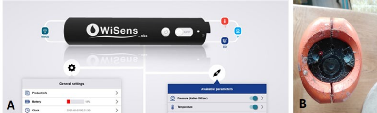
Figure 24: DO sensor's low battery level indication (A) and fouling (B) after 3 months underwater.
