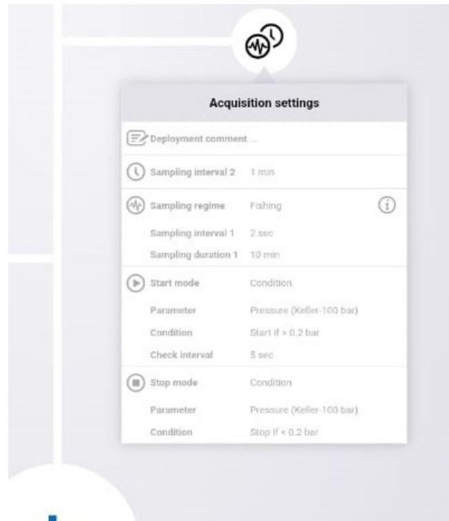
Figure 2: Sensor acquisition settings for the fisheries sampling regime as of 7 July 2023.
