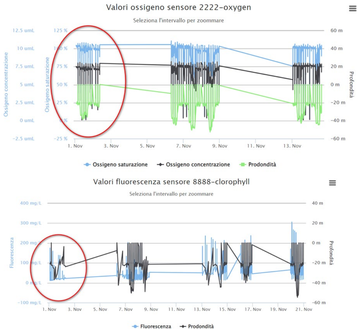
Figure 6: AdriFOOS web viewer shows the hauls recorded in the same period by the DO 2222 (top) and Chl-a 8888 (bottom) sensors in November 2023, highlighting for the latter inconsistent activation behaviour.
