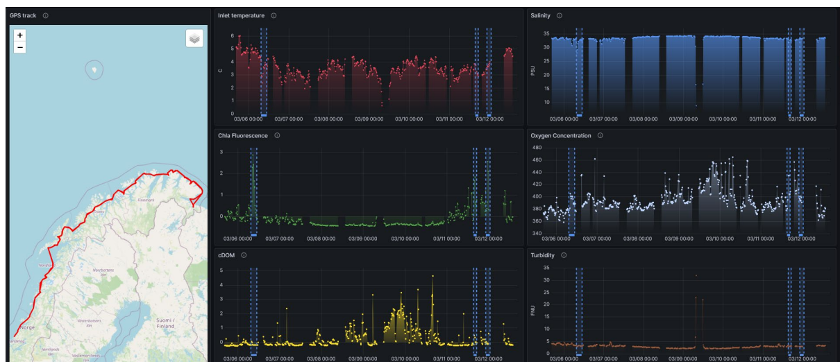
Figure 32: Example of annotation of algae blooms on NIVA FerryBox installed on board of MS Richard With, sailing through a large distance of coast of Norway, between Bergen and Kirkenes.
