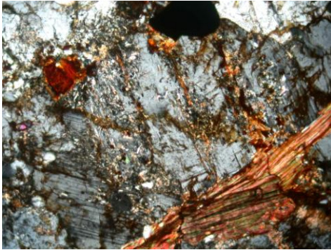
Fig. 3 – Photomicrographs of highly weathered sample (class IV) (10X, crossed polarized light).
