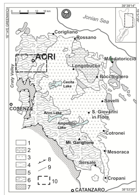
Fig. 1 – Geologic sketch map of the Sila Massif (modified from MESSINA et alii , 1994) with location of the study area. Legend: 1) predominantly clastic deposits (Recent to Tortonian). 2 to 6 = Sila Unit: 2) Mesozoic to Tertiary sedimentary cover; 3) plutonic rocks (Sila Batholith; Carboniferous-Permian); 4) low-grade metamorphic rocks (Bocchigliero Complex; Late Cambrian to Early Carboniferous); 5) low - to medium-grade metamorphic rocks (Mandatoriccio Complex; Late Cambrian to Early Carboniferous); 6) medium-to high-grade metamorphic rocks (Monte Gariglione-Polia-Copanello Complex; pre-Triassic); 7) Lower Alpine thrust nappes of the Sila Massif including Castagna, Bagni and Ophiolitic Units (phyllite + schist and ophiolitic rocks); 8) thrust fault; 9) stratigraphic contact; 10) studied area.
