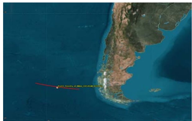
Figure 10. Progress-M 27M JSpOC reentry assessment at 80 km with \pm 1 minute uncertainty
