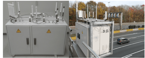
FIGURE 1. RSU equipment: front view of the RSU at the left and its deployment on the highway at the right.
