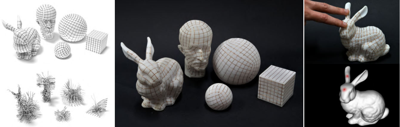
Fig. 1. Our computation fabrication method for multi-touch sensing on general 3D surfaces. (Left) 3D models with grooves to accommodate the touch sensor conductors and the internal pipes to connect the surface lines with the touch controller. (Center) Photo of the 3D printed prototypes equipped with the touch sensor grid made of enamelled unipolar solid copper conductor. (Right) An example of touch interaction with two fingers with the relative positions computed on the 3D model.
