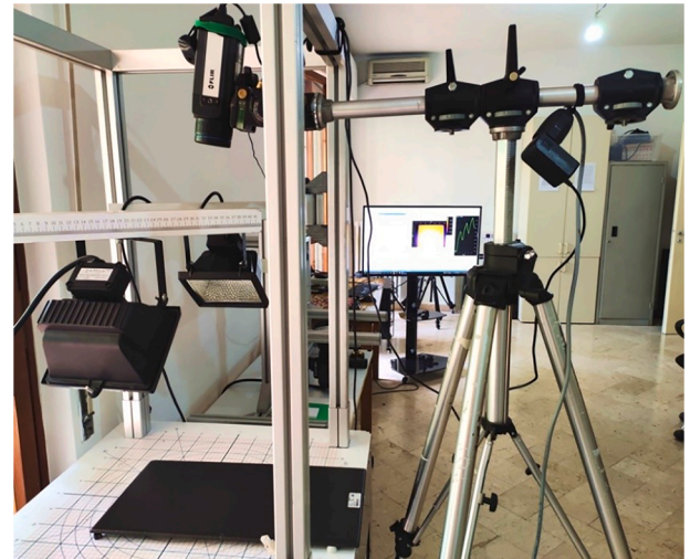
Fig. 3. Experimental set-up. The experimental tests have been carried out by adopting a reflection configuration mode.
