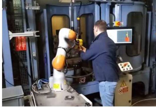
Fig. 31 A LUS upgraded with a robot system for a collaborative version of pallet preparation tasks: the robot system provides services from lateral approach (from left side), sharing the workspace with a single LUS operator (Cortesy of: Cembre SpA, Brescia, Italy).
