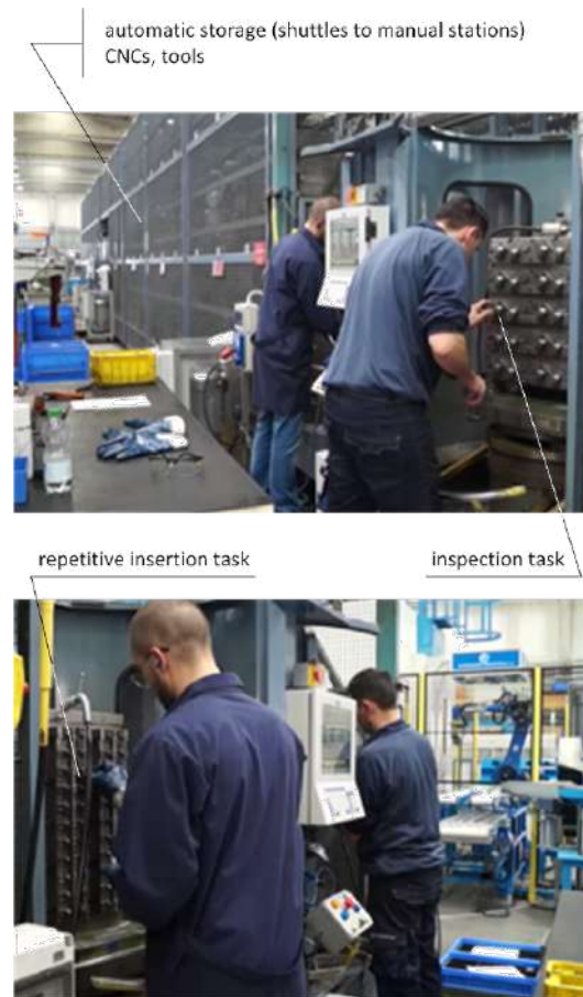
Fig. 30 Production scenario with heavy-duty manual tasks at LUSs (Cortesy of: Cembre SpA, Brescia, Italy).
