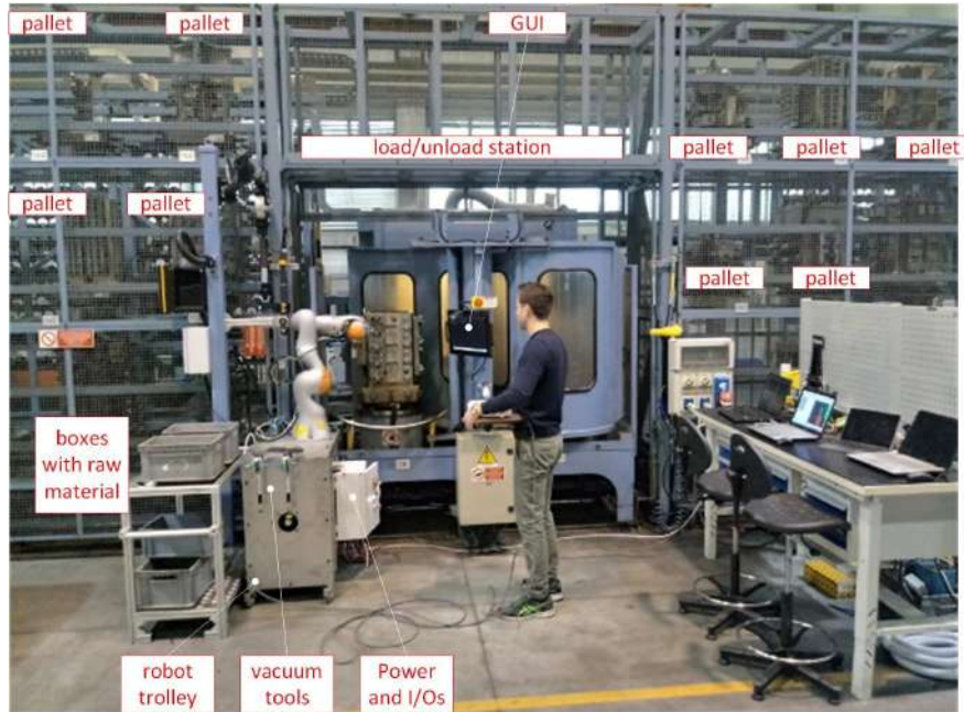
Fig. 37 Frontal view of a LUS including the piROS setup. The LUS is composed of two pallet units, of which only the left side one has been equipped with the robot system. Right hand side unit continues to operate manually (pictured with its sliding doors closed). The robot system is relocated on the left-end side of the left pallet unit (pictured with open doors and a pallet available in the processing area). The LUS, approx. 2300x3100 mm wide and high, is surrounded by the storage unit, where pallet are shelved and shuttled within the FMS. The portion of the FMS not visible in the picture include the full-length storage (approx. 30 m), another manual LUS, the shuttle delivery system travelling behind the LUSs, and 3 CNC machine tools (partially visible in the background, on the opposite side with respect the shuttle track). Notable elements of the system are labelled. (Courtesy of Cembre SpA, Brescia, Italy).
