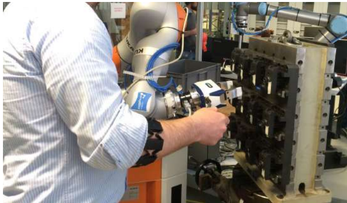
Fig. 39 Example of CNC pallet featuring twelve 2-slot jigs: each part is flipped between individual slots and inserted in pegs (pictured during development stages).
