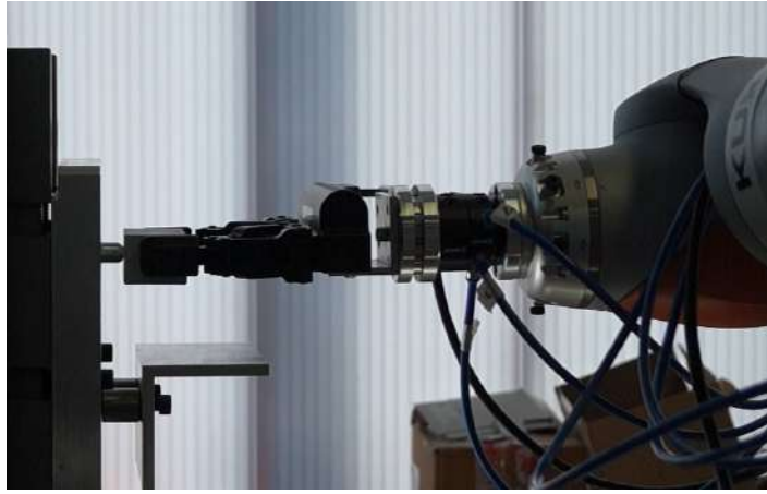
Fig. 41 Example configuration of a fixture assembly task (H7/h6 tolerance).
