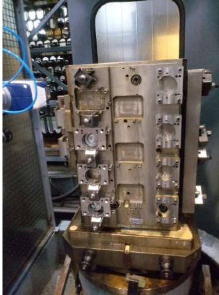
Fig. 32 Example of FMS pallet, with bolts/nuts jigs, inside a LUS during an intermediate machining step: array of parts on left side need to be disassembled and flipped to the right side array jigs for second machining step. Additional different jigs are present on lateral mounting surfaces of the pallet (Courtesy of: Cembre SpA, Brescia, Italy).
