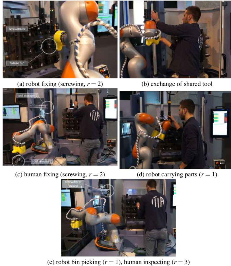
Fig. 34 Example of mixed workflow during an assembly/fixing sub-task (EuRoC field test stage).
