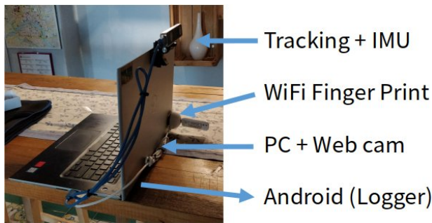
FIGURE 17. The PC-based optical navigation system used during the competition.
