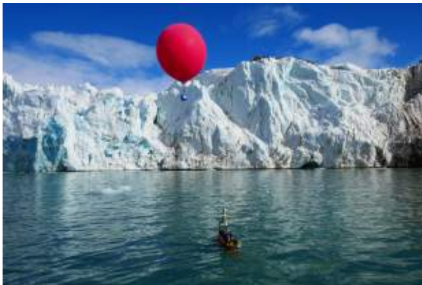
Figure 1. PROTEUS (Portable RObotic TEchnology for Unmanned Surveys) vehicle with atmospheric sensors in the 2018 campaign carried out by CNR-INM in Svalbard.
