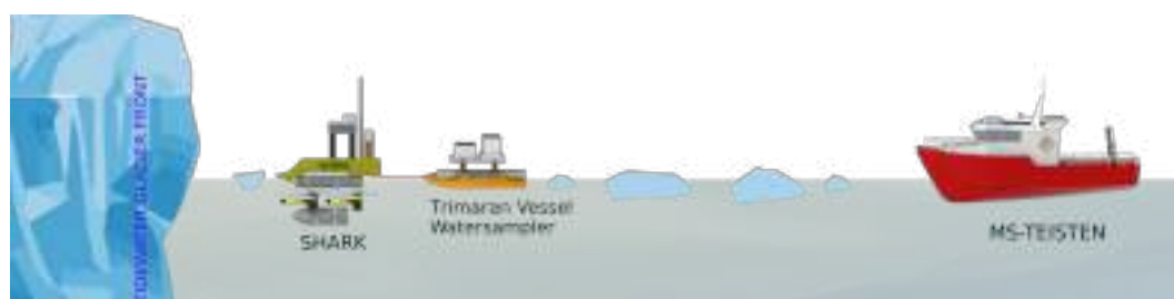
Figure 12. Arctic: Present climatic change and past extreme events (ARCA) project: Shark USSV and towed trimaran (2015).
