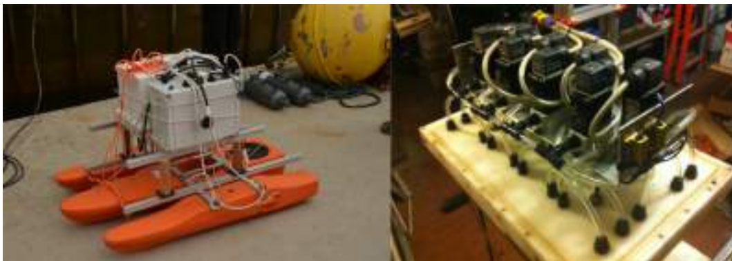
Figure 8. Towed trimaran equipped with an Autonomous Water Sampler (AWS).
