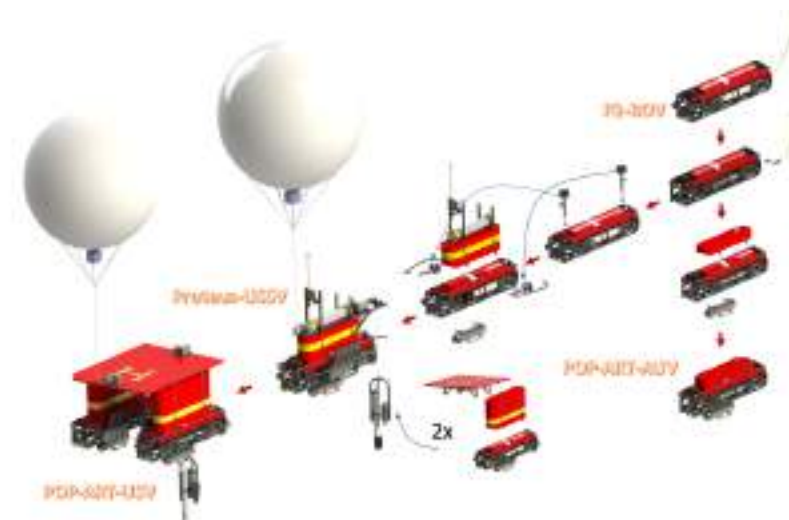
Figure 9. POP-ART (POLar Portable Autonomous Robotic Technology): modular reconfigurable UMV (Unmanned Marine Vehicle) for polar applications.
