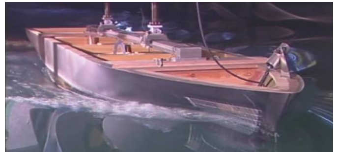
Figure 18. Breaking bow wave during experiments at DGA-Hydrodynamics, Fn 0.328
