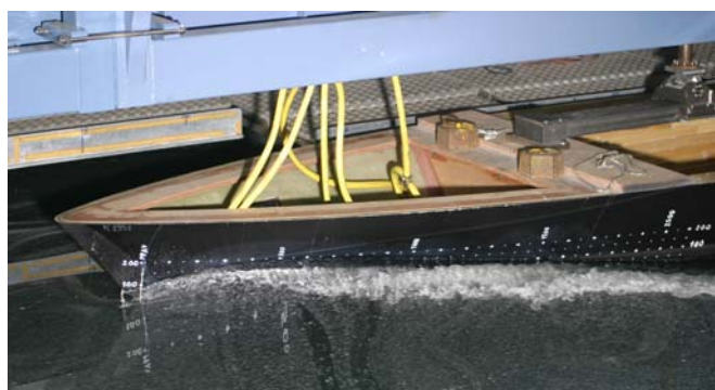
Figure 21. Details of the breaking bow wave during experiments at DGA-Hydrodynamics, Fn 0.328
