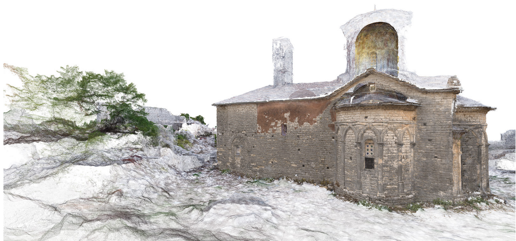
Fig. 9. St. Mary point cloud composed of UAV and close-range photogrammetric survey data.
