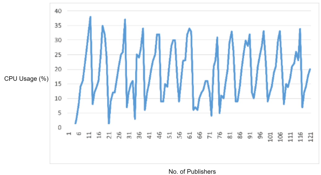
Figure 16. CPU usage captured while performing MQTT DDoS attack when IDS rules are disabled.
