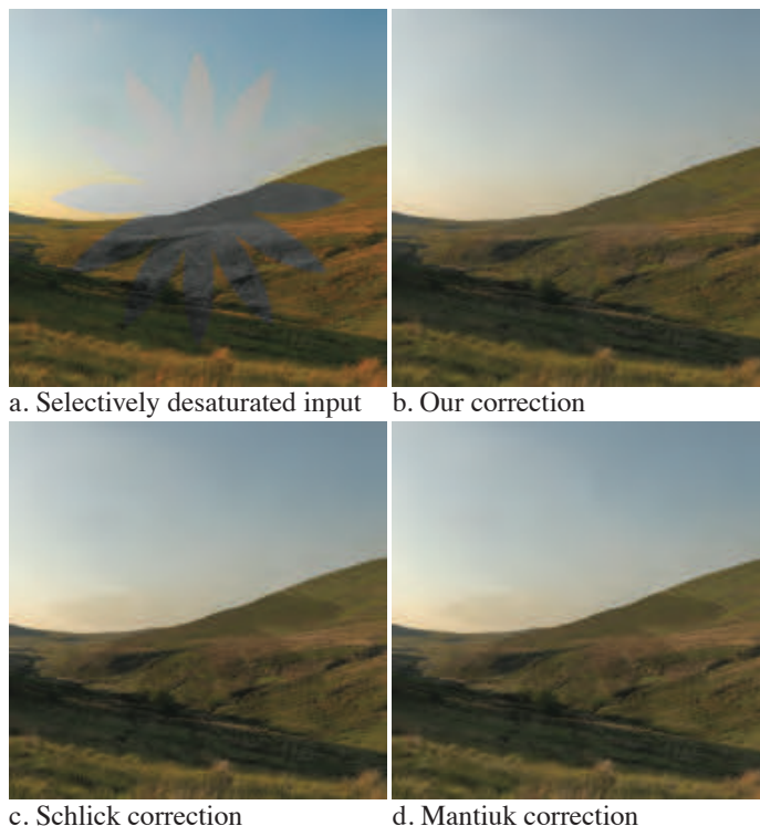
Figure 7: Typically, artists can use masks to control the contrast, saturation and other parameters locally in the image. The input image (a) was manually adjusted using a mask to selectively desaturate the logo, and post-processed with our algorithm (b) as well as Schlick’s (c) and Mantiuk et al.’s [6] (d) corrections.
