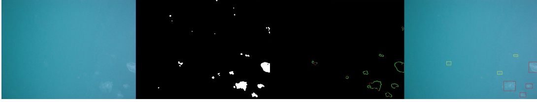
Fig. 2: Feature extraction steps: original image (extreme left), binarized image (center left), segmented image (center right), labeled image (extreme right).
