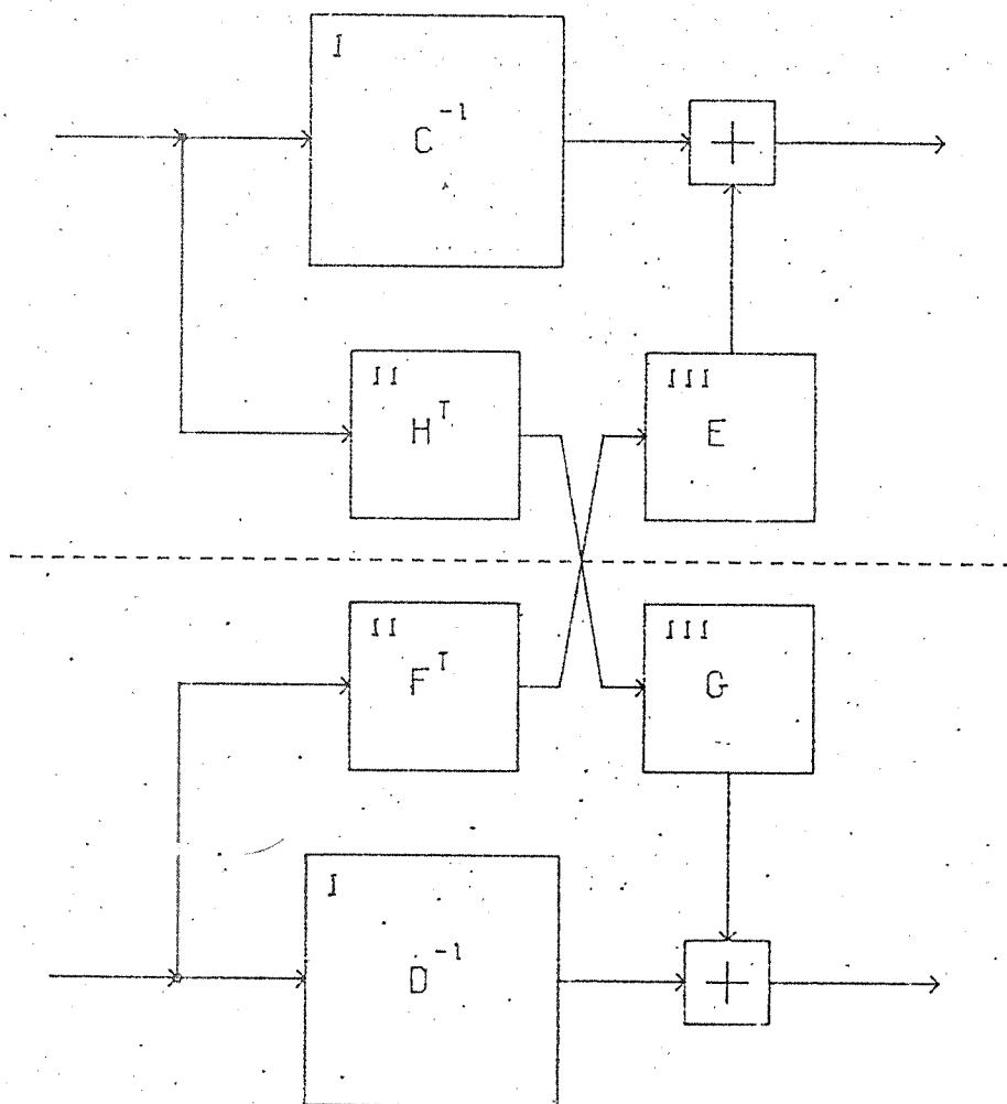
Fig.1 Recursive module structure.
