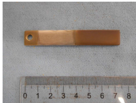
Figure 2. Substrate # 2 with AlN film magnetron sputtered. Moving from right to left: the film is deposited for a length of 35 mm; the following 30 mm were masked, and in the figure the aluminum substrate without film deposition is visible; finally, the film is on the last 10 mm (where a hole is present for connection).
