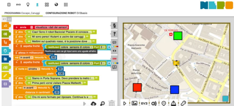
Fig. 4 “X-Scape Carruggi”. This is a snapshot of the OpenRoberta website page created for the “X-Scape Carruggi” activity, in which children are asked to develop an easy program to move a robot from the archeological site at Giardini Luzzati in Genoa, Italy (highlighted as a red square on the map) to the closest subway station (highlighted as a green square)
