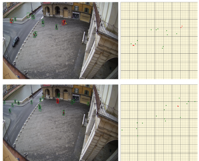
Figure 5: Examples of the output of our social distance measurer module. Left: images with the detected pedestrians. Right: 2D projection on a virtual planar surface obtained through homography. Green color means a safe placement; red color indicates violations of the social distance rule. Image Courtesy of [Di Benedetto et al. , 2021].
