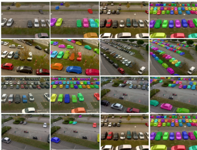
Figure 1: Examples of the output of our vehicle counting solution. We show input images captured by smart cameras and the detected vehicles by our CNN-based technique.
