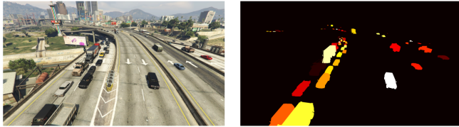
Figure 3: Sample of our GTA dataset. It is the first synthetic dataset of urban scenarios where per-pixel annotations are automatically gathered from a virtual-world.
