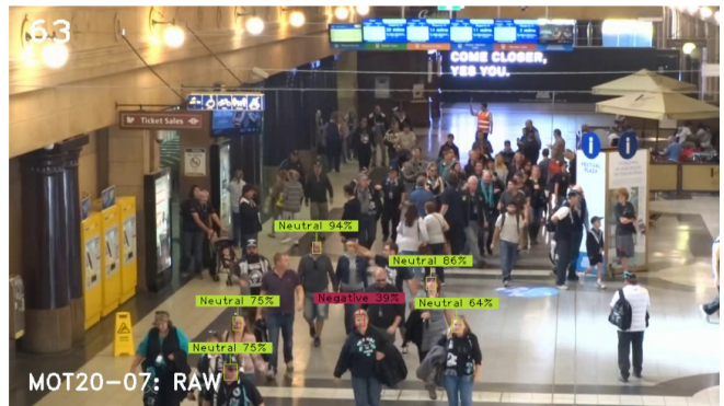
Figure 4: Example of the output of our Facial Expression Recognition system. We recognize human facial expressions by automatically analyzing images.
