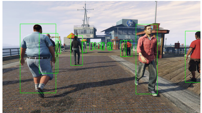
Figure 2: Sample of our ViPeD dataset. Images and bounding boxes localizing the pedestrians are automatically gathered from a virtual-world. Image Courtesy of [Ciampi et al. , 2020b].
