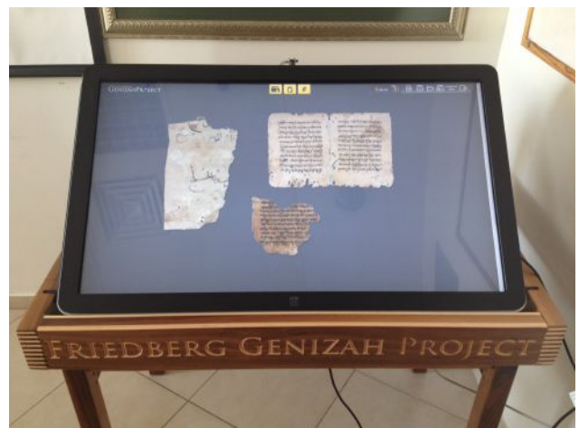
Fig. 5: The large touch screen mounted on a specially designed chasis, showing the fragment at hand together with 2 suggested joins.
