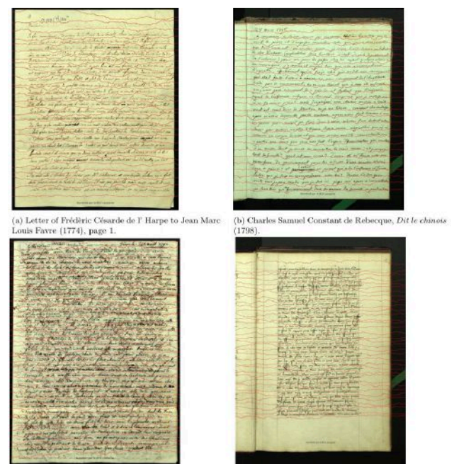
Fig. 10: Seam carving results on manuscripts of the 16-th and 18-th century respectively. Even in the lower left manuscript with extreme bleed-through, our algorithm is able to produce a robust result.
