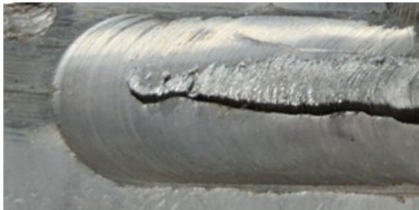
Fig. 6. Particular of the FSW joint surface made with Tool n. 3.
