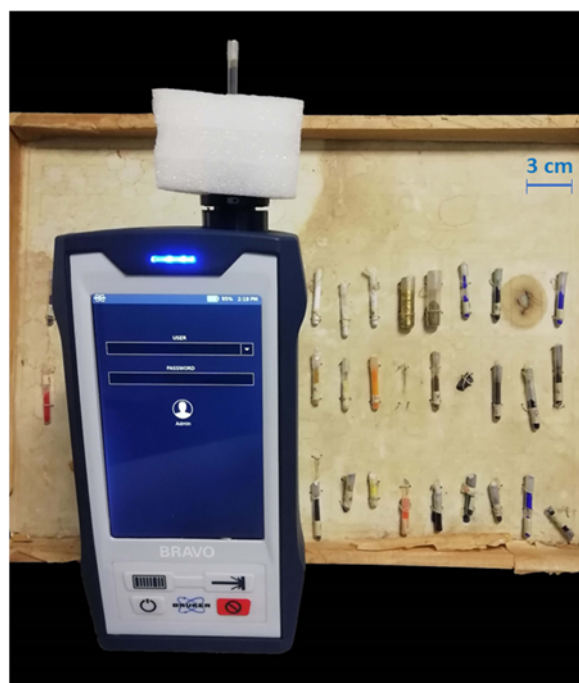
Figure 2. Set-up of pSSE Raman measurement of pigments inside the glass vials placed in the laser beam.
