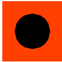
(c) Chamfer distance with 24 adjacent pixels per node ( 5 \times 5 square centred on node).
