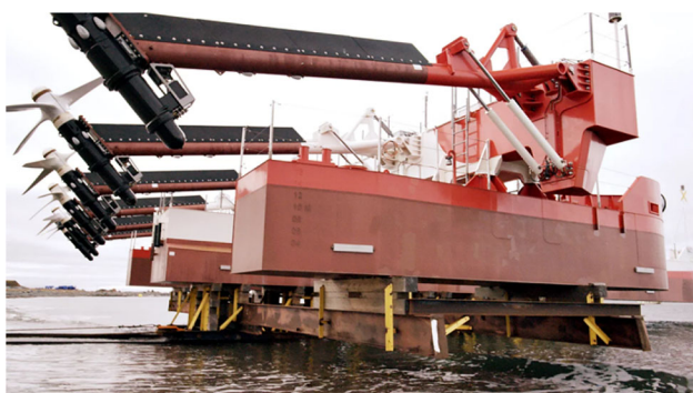
Fig. 1 Schottel hydro-SIT turbines installed on the Sustainable Marine Energy platform PLAT-I 6.40
