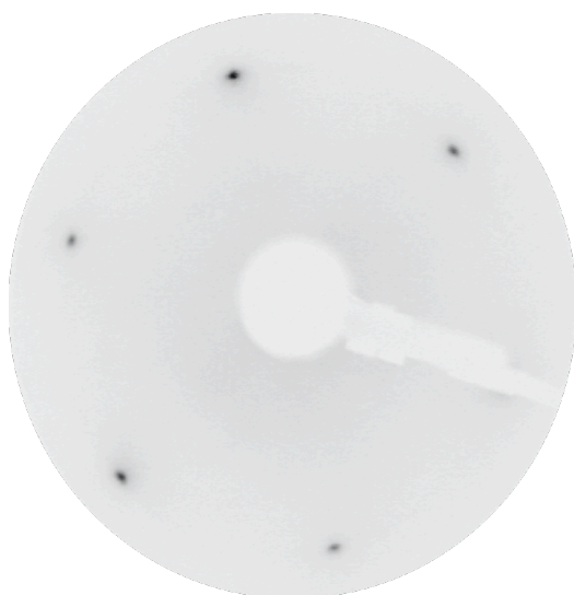
Figure S2: LEED pattern of N-Gr/Ni(111), showing the (1x1) structure of epitaxial Gr ( E = 70 eV)
