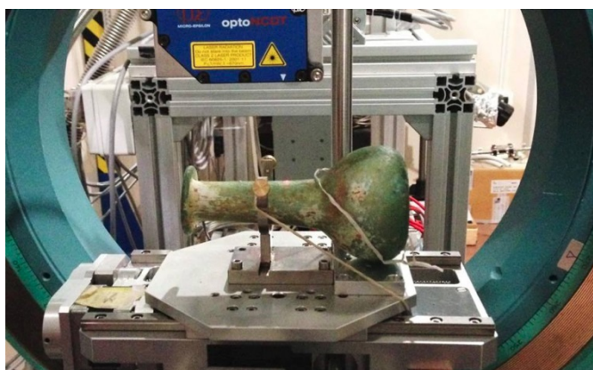
Figure 1. The diffractometer, equipped with the laser interferometer, hosting an object relevant for cultural heritage for x-ray diffraction analysis.
