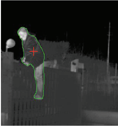
FIGURE 7: Example of an identified and segmented person during video surveillance on a gate.
