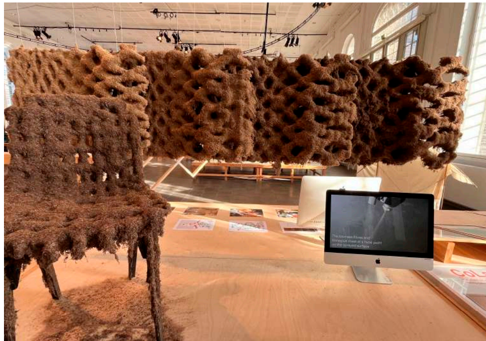
Figure 16. Prototype of a “3D sprayed” chair, developed at Center for IT in Architecture—CITA, Copenhagen, DK. Photo by Giuliano Galluccio.
