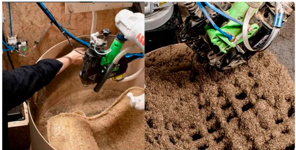
Figure 17. 3D spraying process, developed at Center for IT in Architecture—CITA, Copenhagen, DK. Photo by Giuliano Galluccio.
