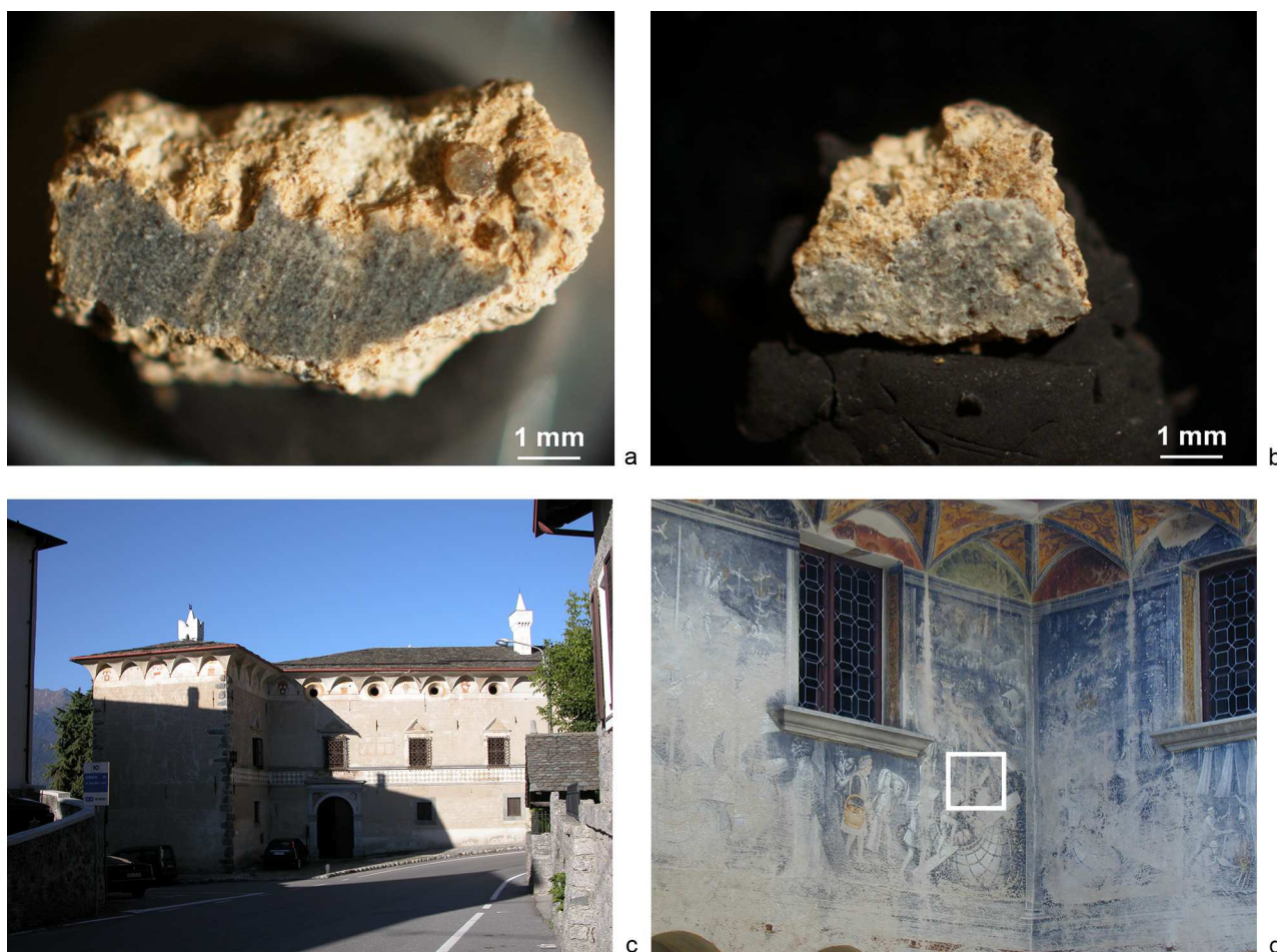
Figure 1. PB50 (a) and PB52 (b) fragments used in micro-SORS measurements; Palazzo Besta (c) and detail of the painted façades of the internal court with indication of the sampling area (white square) (d).
