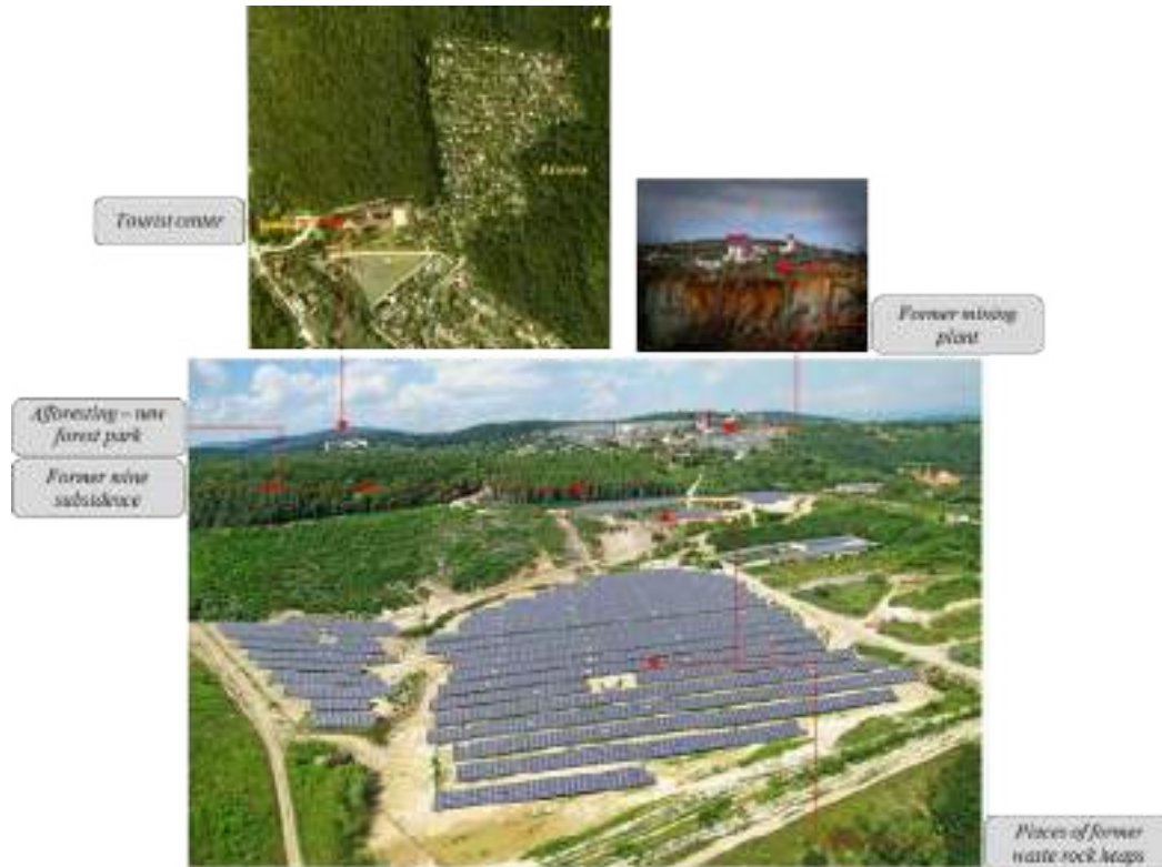
Figure 7. Subsidence and surrounding (Košice-Bankov) after reclamation (2016). Solar collectors in the places of the former waste rock heaps; afforestation (in the background) in the place of the former subsidence.
