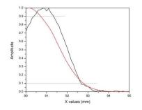
pixel in the image. In Fig. 1 it is shown the improvement in spatial resolution of a sharp metallic edge imaged in transmission mode at 0.3 THz due to the knife-edge technique. The maximum slope of each profile was calculated between 0.1 and 0.9 of the maximum intensity finding that without the blade amounted to 0.44/mm, whereas with the blade, the slope reached 1/mm, with an enhancement of 2.3 times.
