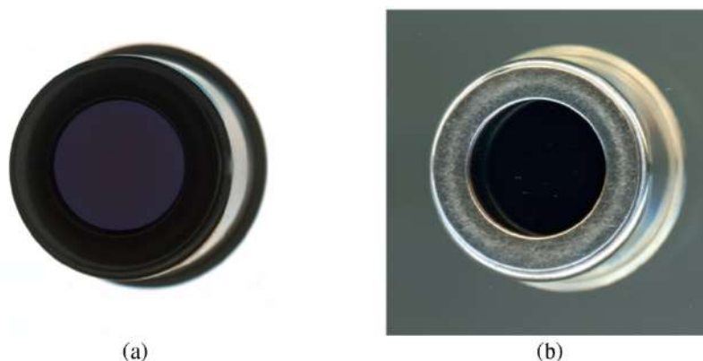
Fig. 2 Optical scan in transmission (a) and in reflection mode (b) of a typical sample mounted on a TO-8 standard frame with 7 mm clear aperture diameter.
