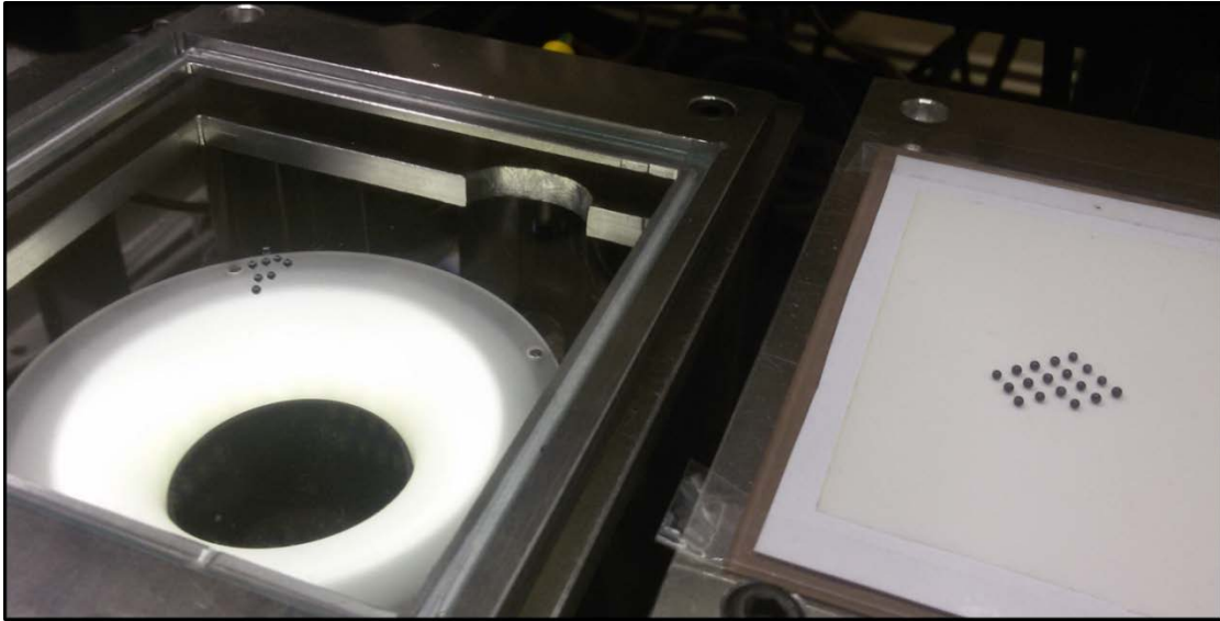
Fig. 7. Calibration of the second camera. On the left, the -area1 used as a gripping area seen by the first camera; on the right, the -virtual grid is in under construction in area2.
