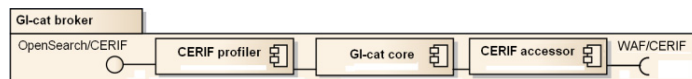
Fig. 3 The two new GI-cat components: CERIF profiler and accessor, designed to support CERIF data model in the GI-cat brokering framework.
