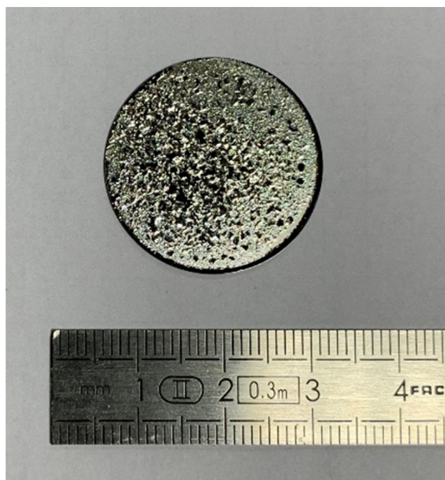
Figure 8. Picture of sample S7W after 16 keV proton irradiation with a fluence of 10 17 cm -2 .
