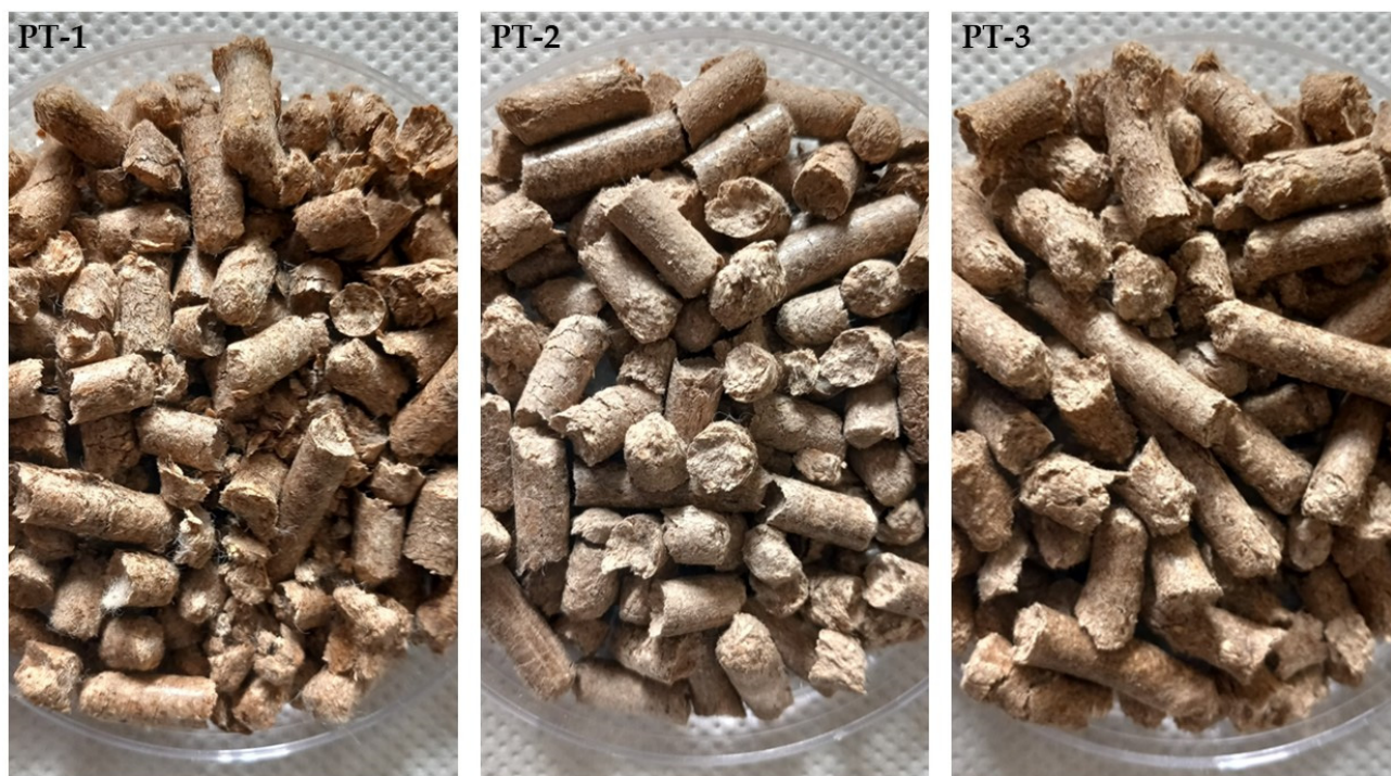
Figure 2. Pellets produced by the three tests: (PT-1) ratio spruce sawdust: wool = 1:1; (PT-2) ratio spruce sawdust: wool = 2:1; and (PT-3) ratio spruce sawdust: cut wool = 2:1.
