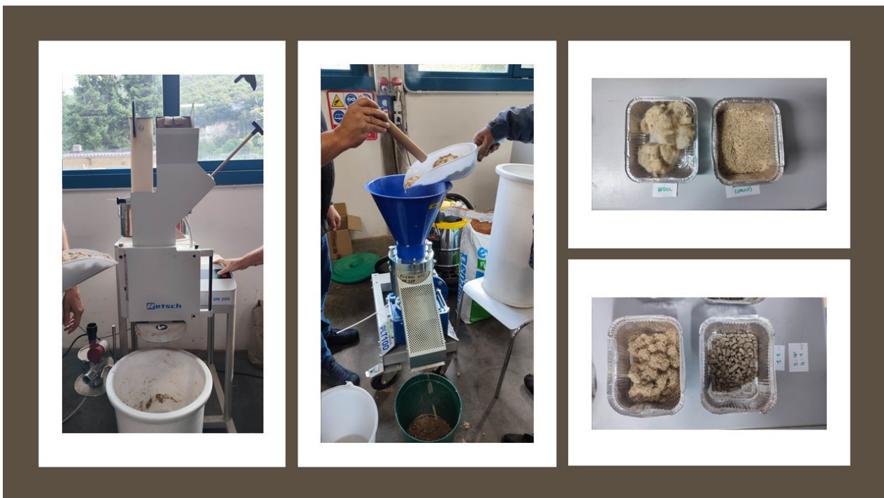
Figure 1. Cutting mill on the left and pellet machine at the center . Up on the right , the matrices: wool and sawdust. On the bottom right , an example of mixture (1:1) and pellets (1:1).
