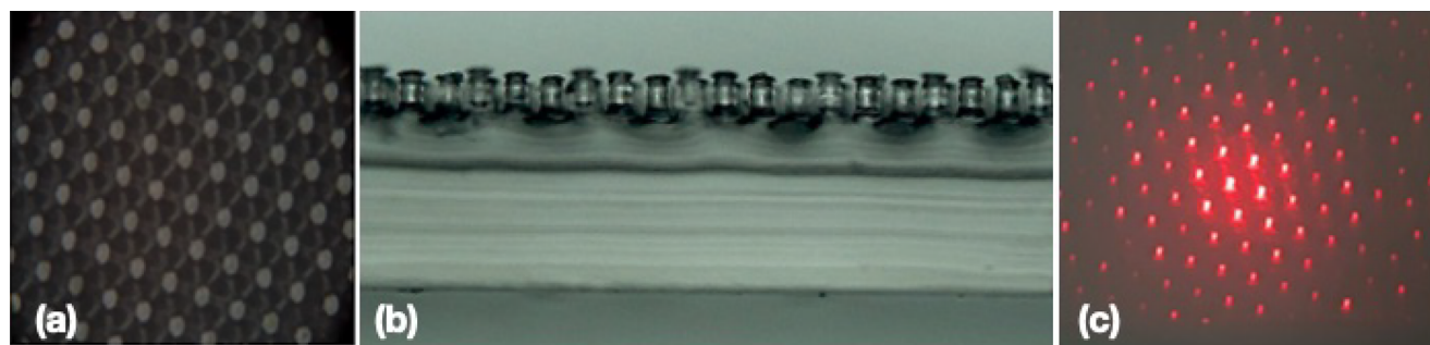
Figure 6. Micrographs taken by a standard optical microscope in transmission (a) with 20 \times magnification of the surface and (b) the cross-section of GT. (c) Transmission diffraction pattern produced on a screen by a red laser pointer shone through the sample.
