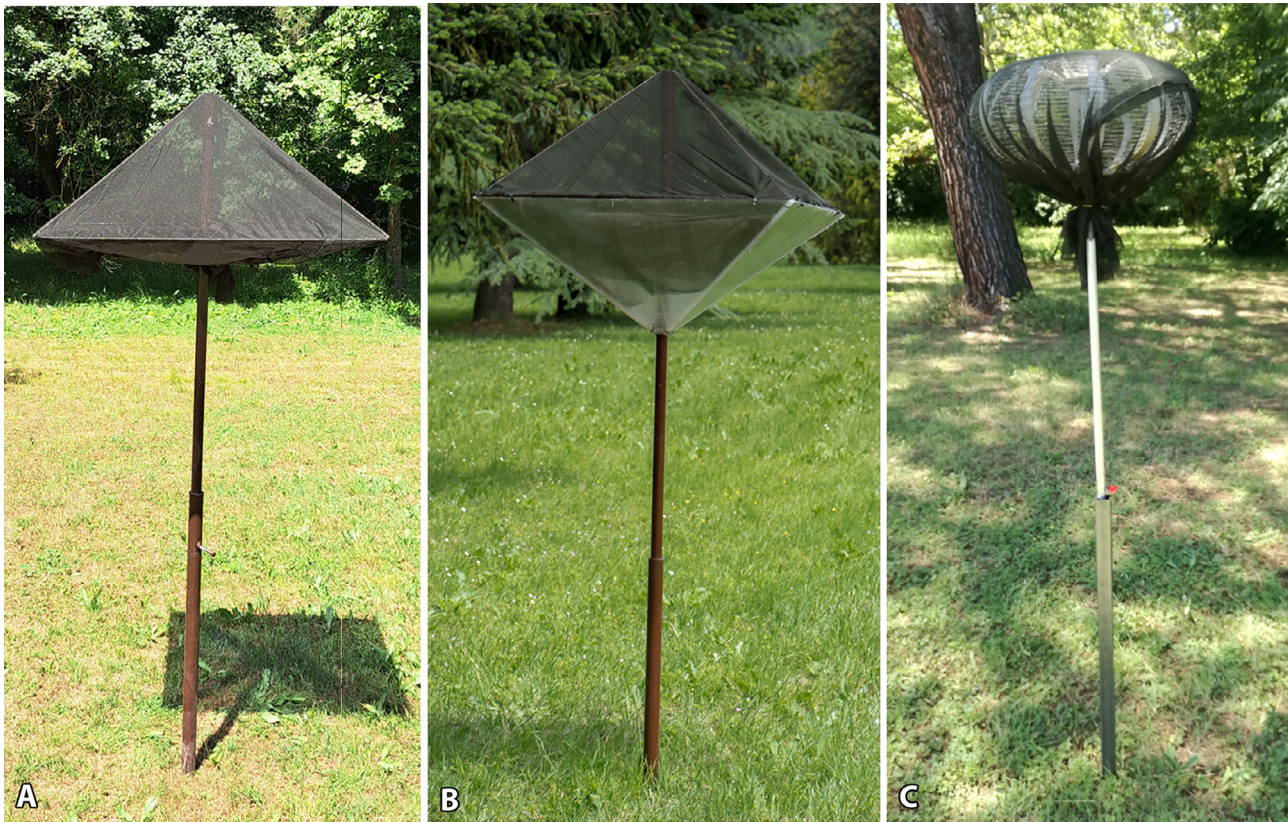
Figure 2. Different forms of attract-and-kill devices (A&Ks). A: pyramidal A&K. B: octahedral A&K. C: ellipsoidal A&K.
